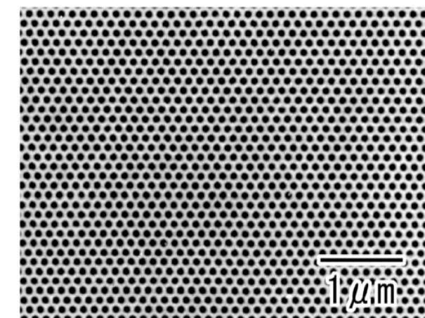
**Fig. 1.** SEM image of the surface view of the ideally ordered anodic porous alumina.
