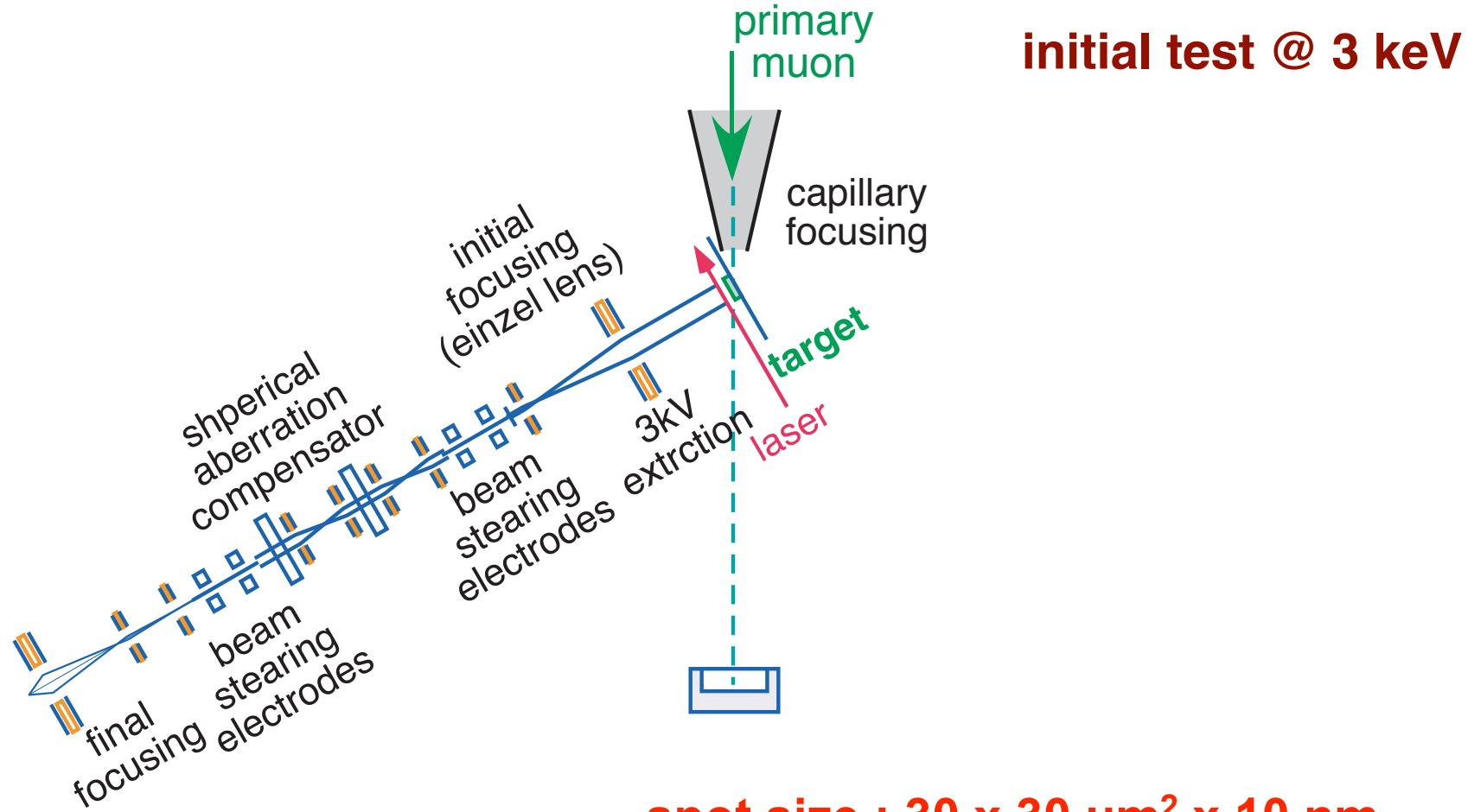
spot size :  $30 \times 30 \mu\text{m}^2 \times 10 \text{ nm}$
