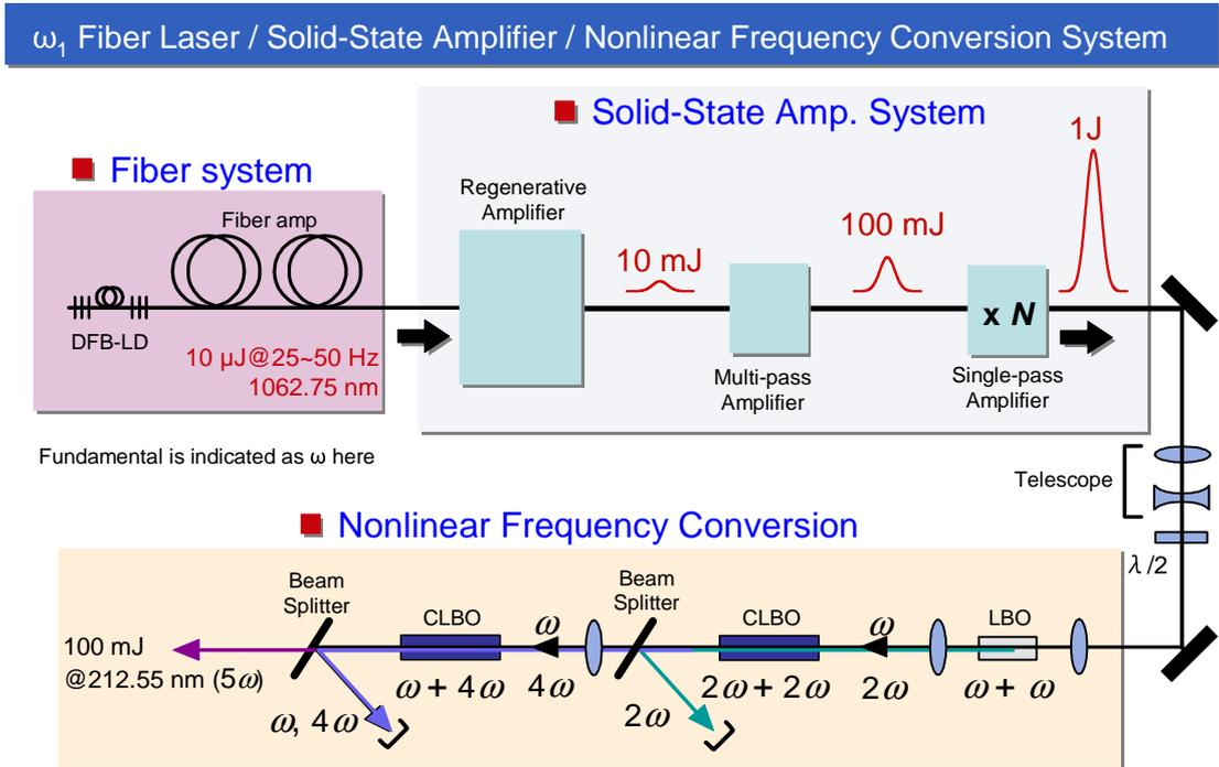
FIG. 25: laser system for generating  $\omega_1$ , 212.55 nm
