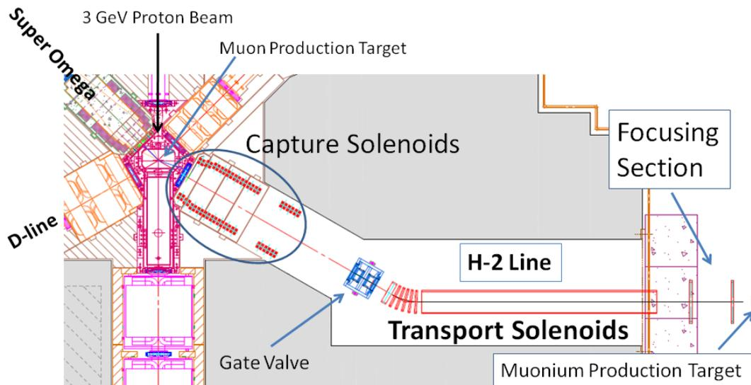
FIG. 15: Schematic picture of the H-2 beam line.
