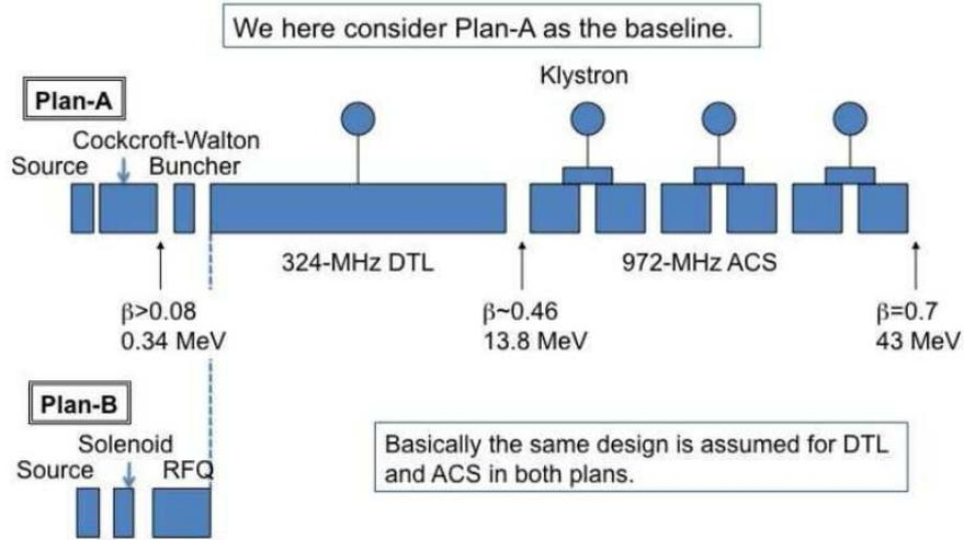
FIG. 28: Schematic layout of low- $\beta$  linac.
