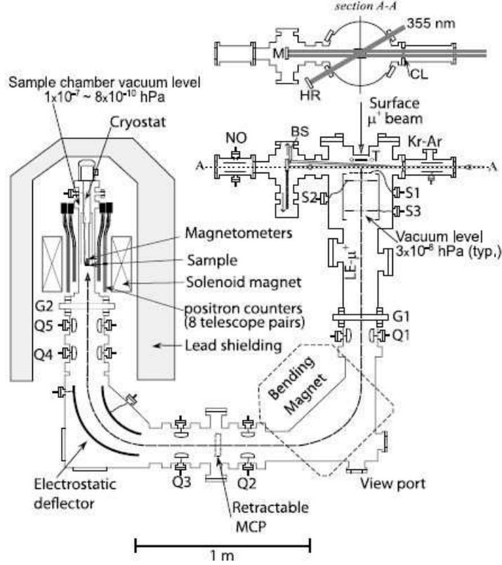
FIG. 18: A experimental layout of the slow muon beam line at RIKEN-RAL muon facility
