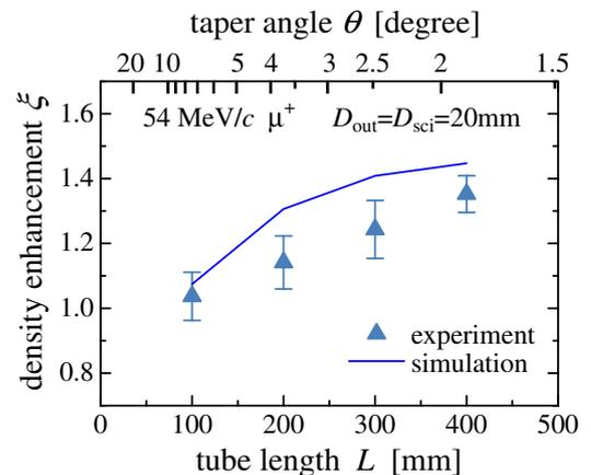
Fig. 4. (Color online) The beam density enhancement  $\xi$  for 54 MeV/c  $\mu^+$  as a function of the tube length  $L$  for  $D_{out} = D_{sci} = 20$  mm. The solid line shows the simulation.
