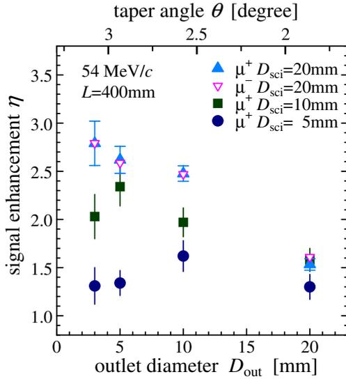
Fig. 2. (Color online) The signal enhancement factor  $\eta$  as a function of outlet diameter  $D_{out}$  for 54 MeV/c muons with  $L = 400$  mm tubes for  $D_{sci} = 5, 10,$  and  $20$  mm. The error bar includes statistical and systematic errors (see text). Data points with “T” shape error bar are the mean of multiple measurements and those with “|” shape error bar are measured only once. Error bars of  $\mu^-$  data are omitted for clarity.
