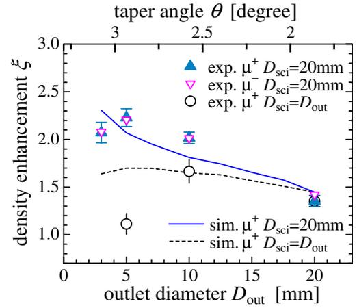
Fig. 3. (Color online) The beam density enhancement  $\xi$  for 54 MeV/c muons as a function of  $D_{out}$  for  $D_{sci} = 20$  mm and  $D_{sci} = D_{out}$ . The solid and dashed lines show the results of the simulation for  $D_{sci} = 20$  mm and  $D_{sci} = D_{out}$ , respectively.
