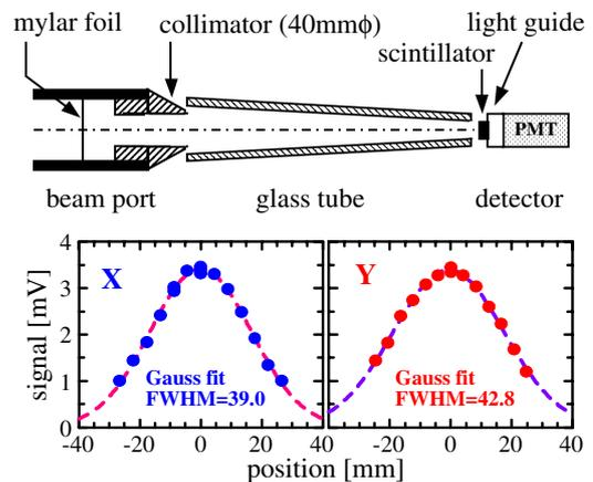
Fig. 1. (Color online) Top: a schematic view of the experimental setup (not to scale). Bottom: the beam profile of 54 MeV/c  $\mu^+$  measured with a 5 mm $\phi$  scintillator positioned 403 mm downstream from the collimator.
