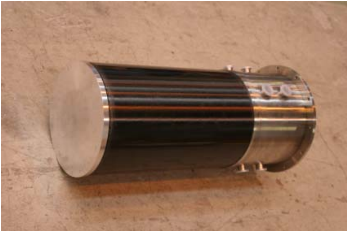
(4) Fabrication and assemble of CFRP vacuum pipe and 8 18pin-connectors
