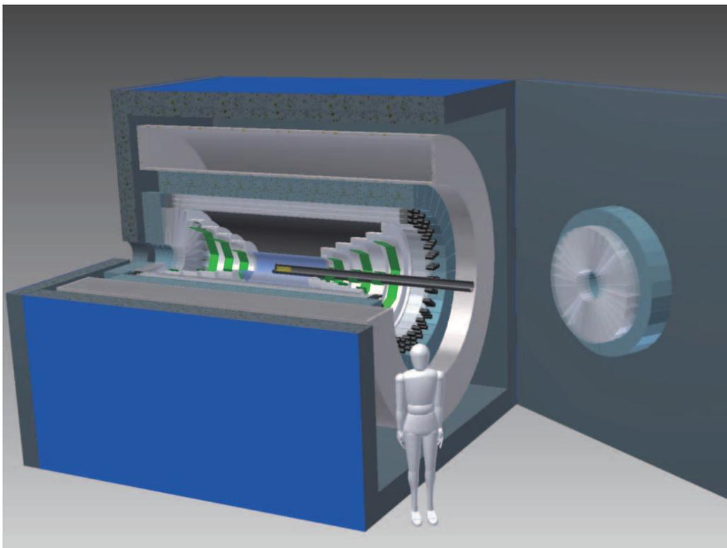
Figure 3: Conceptual design of the new CDS.
