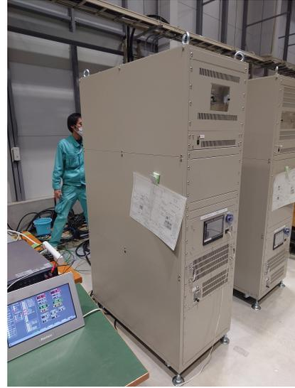
Figure 27: Power supply for the superconducting solenoid magnet.
