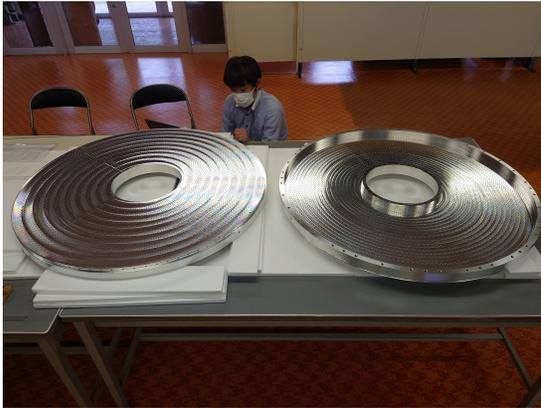
Figure 51: CDC endplates machined by SEIRITSU CO., LTD.
