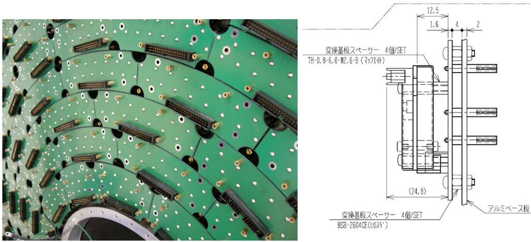
Figure 50: Existing signal boards placed directly on the end plates of the CDC and its design. We use the same designed boards for the newly constructed CDC.
