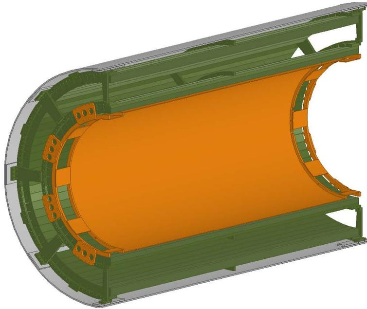
Figure 70: Structural calculation model. The constraint condition is the end face of the inner cylinder of the magnet, and the parts are glued together. A gravity of 2 G is applied from the vertical direction.
