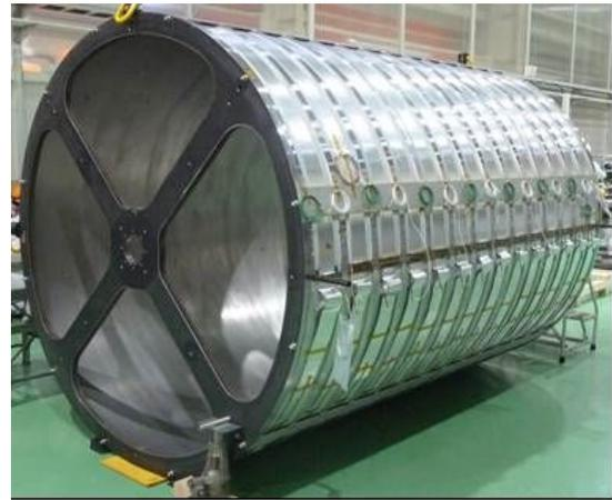
Figure 17: Photo of the superconducting coil completed in March 2024.
