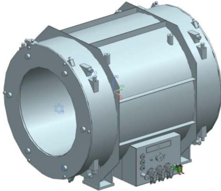
Figure 21: Schematic view of the vacuum vessel. Support structures for the detector system, vessel reinforcements, etc. on the inner wall are not shown.
