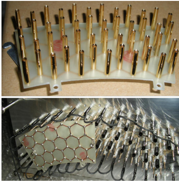
Figure 2: H.V. distribution board prototype connected on CDC prototype for test
