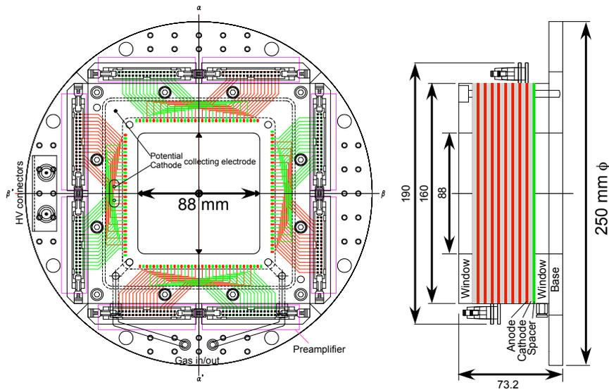
Figure 17: A design drawing of VBLC
