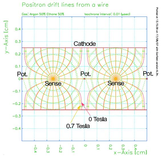
Figure 19: Drift lines from a wire (calculated with GARFIELD)
