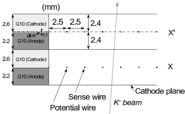
Figure 18: A schematic illustration of a cross section of the VBLC
