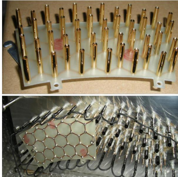
Figure 8: H.V. distribution board prototype connected on CDC prototype for test
