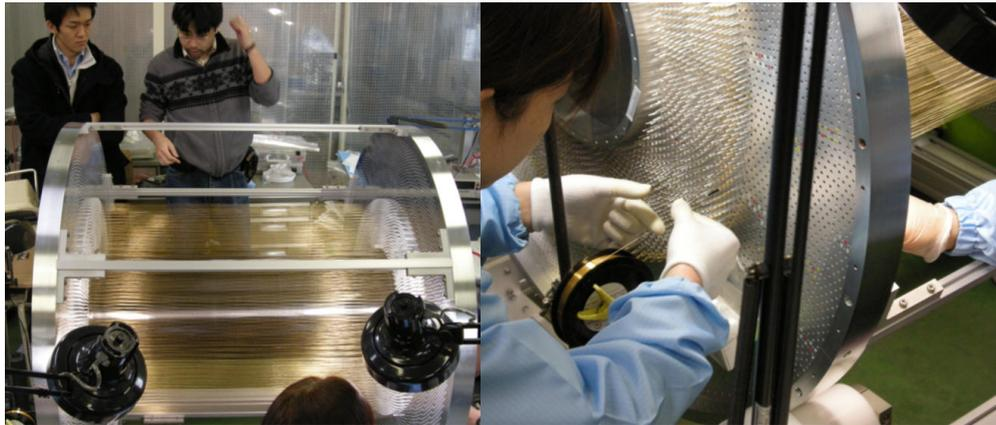
Figure 11: Construction of the CDC at factory
