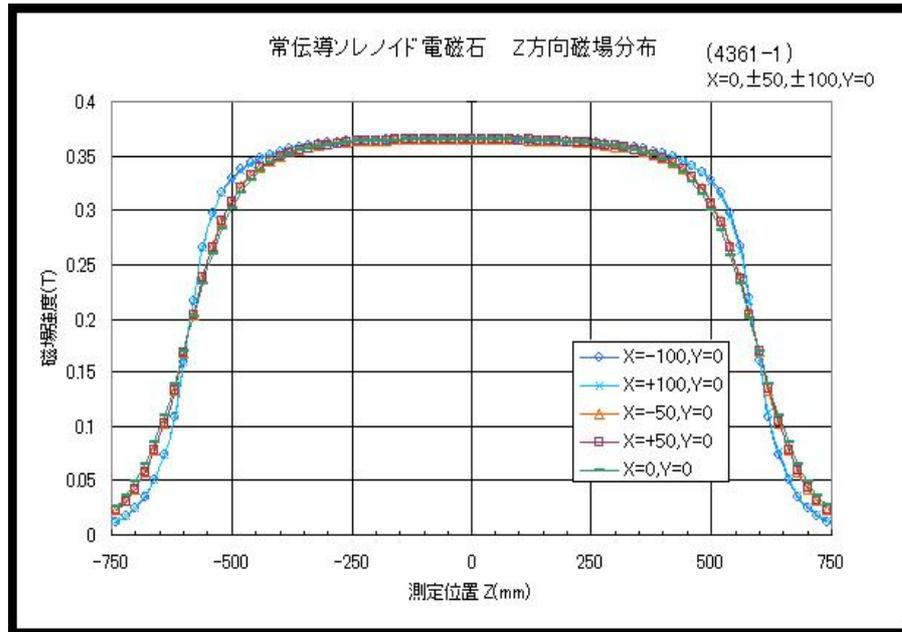
Figure 5: Measured field strength inside the solenoid magnet along the beam direction.
