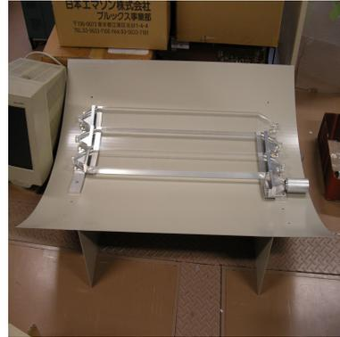
Figure 13: test modules of CDH with dummy solenoid magnet
