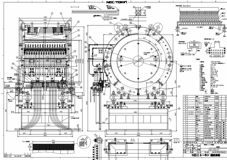
Figure 3: Design for solenoid magnet
