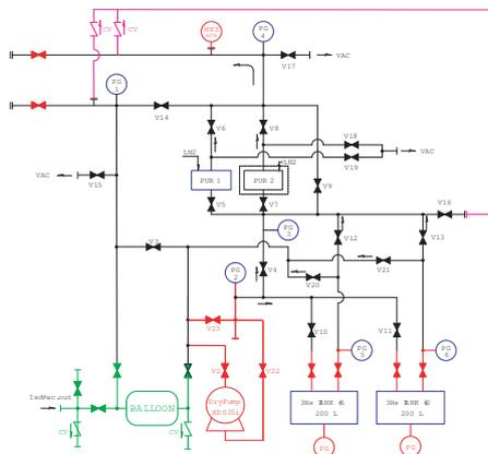
Figure 15: Schematic view of gas handling system
