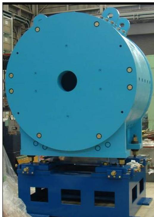
Figure 4: E15 solenoid magnet
