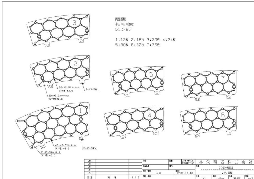
Figure 9: Design of H.V. distribution board
