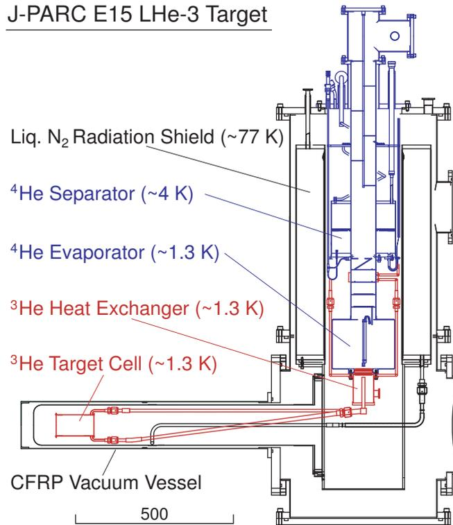
Figure 14: Design of  $^3\text{He}$  target cell
